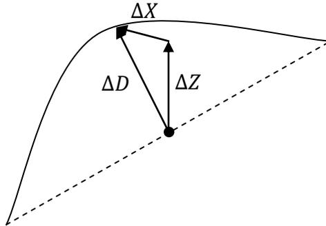
The length of the trailing edge before any displacement was 12 feet, or 3.658 meters. After the final iteration, it was 3.688 meters (calculated by adding up the length of the line segments between all points on the trailing edge). This is an extension, or stretch, of the trailing edge by  $(3.688 - 3.658) / 3.658 = 0.82\%$ .
