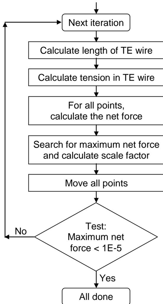
Changes to the main procedure, in module BuildKite.vb, are summarized in the flow chart to the left. The length and tension of the trailing edge wire is calculated at the start of every iteration. Then, as before, the net forces acting on all grid points is calculated. The point subjected to the greatest net force is allowed to move a preset distance (stored in variable MaxAllowedMove), and a scale factor is used to move all other points a distance in proportion to the net forces acting on them.
