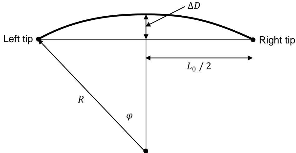
The radius  $R$  of the generating circle (each row in the grid of points will have its own radius  $R$ ) can be derived from the Pythagorean Theorem:
