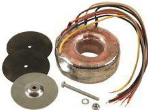
When the primaries are wired in parallel and the secondaries are wired in series, it provides 44Vrms at 3.64A. What is interesting is that it is a toroidal transformer. I had never used toroidal power transformers before and was impressed. They are truly beautiful to look at. They are compact and can be mounted on the walls of the enclosure.
