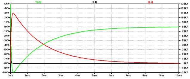
The armature current is a nice single pulse. The barrel coil current is nice, too. It declines steadily from 10KA to zero, with no overshoot. Not so nice is the voltage over the capacitor. The capacitor discharges very quickly, and then continues to charge up in the reverse direction, reaching twice the reverse voltage that it had originally. This capacitor would have blown itself up after a few microseconds. But, let's put that issue aside for now.
