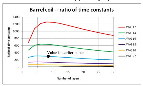
Barrel coil #1 used in the earlier paper has a time constant ratio of about 300 – it is no surprise to us now that the circuit oscillated.
