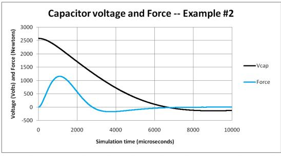
Because the time constant ratio is still greater than 0.25, we would expect to see, and do see, a bit of oscillation remaining. Both the barrel coil's current and the capacitor's voltage make only minor excursions into negative territory.
