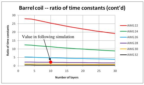
Equation (23) is not the only determinant of oscillatory behaviour, so the 0.25 value is not the end of the story, but it does look as if we are going to be stuck using wire gauges AWG #26 or higher.
