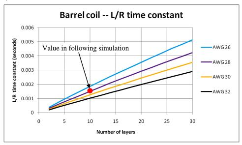
The issue which is going to make this graph important is the speed of the armature. Since the armature will be starting up from rest when it is under the influence of barrel coil #1, it will spend more time in and near barrel coil #1 than any of the other barrel coils further down the barrel. As the armature picks up speed, it will spend less and less time under the influence of each successive barrel coil.
