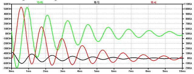
Not only is the energy not delivered in a single pulse, but the voltage to which the capacitor is subjected is simply outrageous.
