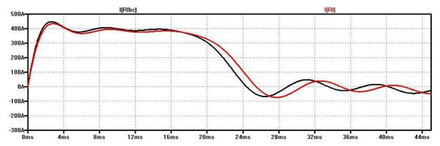
The impact of the change on the load current is modest – the length of the pulse increases by about 1 ms, or approximately 4%. I am happily surprised. I had thought that a five-stage network needed to be well balanced or, stated differently, that it would be very sensitive to the component values. This does not seem to be the case.
