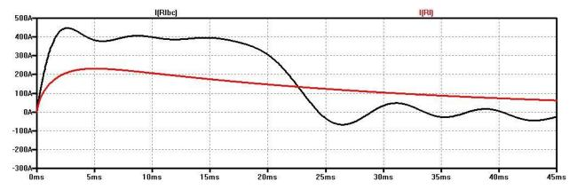
The effect of the equivalent series resistance is much more serious than the previous variations. Not much is left of the pulse. If the ESR per capacitor can be kept at the low end of the range – so that the ESR of the composite capacitor is  $0.1\Omega$ , just equal to the load resistance – then the waveforms look like the following.
