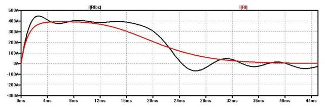
The pulse in this graph is closer to the original one, and may be acceptable for some applications. The lesson here is that the equivalent series resistance of the load capacitors should be as low as possible, and at least less than the value of the load resistance, for the pulse forming network to be able to deliver a discernable pulse.
