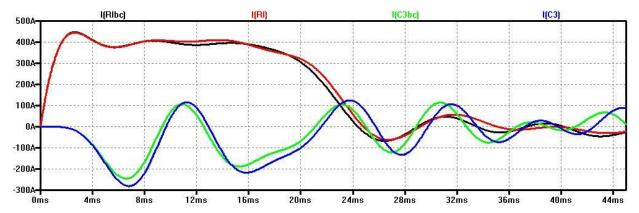
The waveform in black is the "base case" current through the load resistor, where the "base case" is the ideal configuration plotted above. The waveform in red is the current where  $C_3$ 's capacitance is 0.022 F rather than 0.02 F. Indeed, the pulse is very slightly greater and slightly longer.
