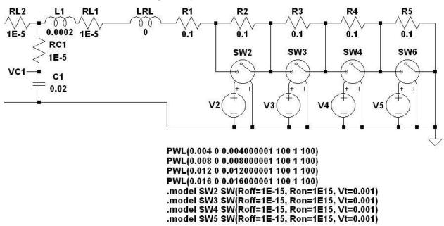
Taken together, the load is a step resistance:  $0.1\Omega$  for the first 4 ms,  $0.2\Omega$  for the second 4 ms, and so on, rising to  $0.5\Omega$  after 16 ms, where it remains.
