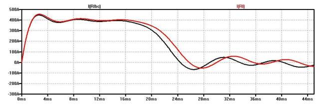
As before, the black waveform is the base case current through the load and the red curve is the load current with the revised component values. While the increase in the length of the pulse is greater for a ten percent change in the capacitances compared with a ten percent change in the inductances, it is still
