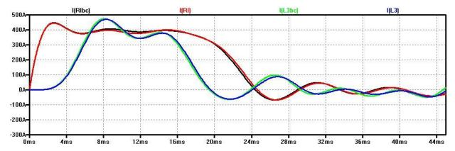
The waveform in black is the base case current through the load resistor. The waveform in red is the current where  $L_3$ 's inductance is increased from 200 mH to 220 mH.
