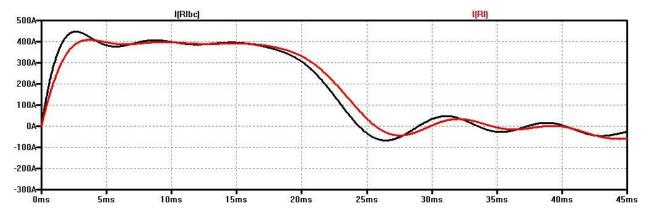
The effect on the pulse is modest and, generally, is a lengthening of the pulse.
