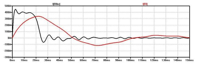
Of course, a condition where the load has an inductance of 2 mH is probably not unexpected. The designer always has the option of using the inductance of the load as all or part of the first-stage inductance  $L_1$ . If the load inductance is known, the choice of the capacitances and the inductances for the network could be made with that in mind.
