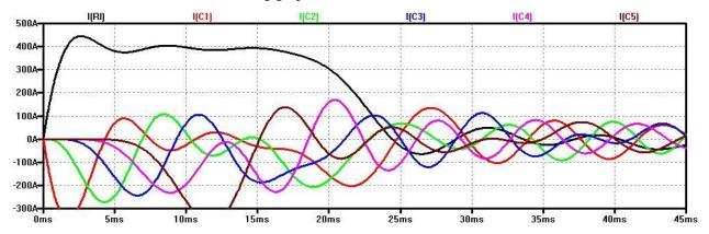
The waveform in black is the current through the load resistors. It can be seen that the capacitors take turns powering the load, in the order  $C_1$ ,  $C_2$ ,  $C_3$  and then  $C_5$ ,  $C_4$ .
