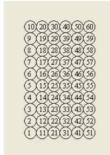
I have not shown the batches in color. Inspection shows that the best positioning is obtained when the leading turn is surrounded by nine additional turns. After that, the next ten best locations describe a second flat coil behind the first. The next best ten locations after that describe a third flat coil behind the second. And so on.
