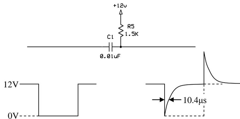
I have shown voltage waveforms below the input and output lines of the R5-C1 pair. The voltage on the input line will go from high-to-low when the slug interrupts the light path. At some later time, when the trailing edge of the slug moves out of the optical slot, the voltage will return high.
