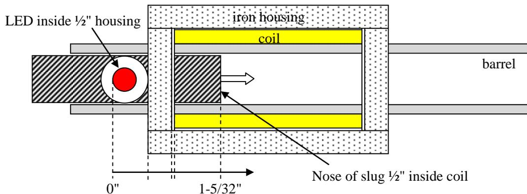
The earliest we could trigger the coil is when the leading edge of the slug passes the upstream edge of the LED, which is the left-hand side of the red circle which represents the light path. The latest we should trigger the coil is when the leading edge is 1/2 inch inside the turns of wire, which is the position of the slug
