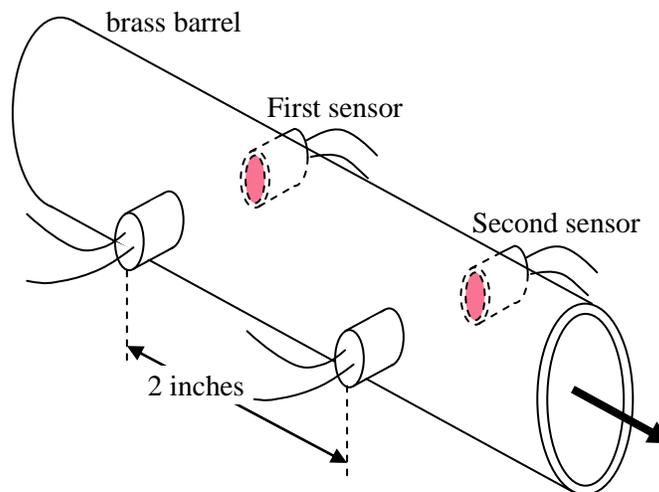
As with the earlier circuit, it is not essential that the sensors and the processing circuit be "fast". It is much more important that they operate in the same way, and introduce the same delay when starting and stopping the timer.
