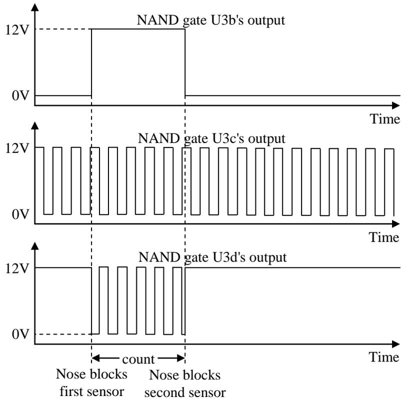
The rising and falling edges of the permission window will not necessarily happen at the very same time that the crystal's 1MHz clocking pulses are changing state. It follows that there will be uncertainty of up to one-half pulse at the start of the window and another one-half pulse at the end. Whatever the count turns out to be, it could be one pulse, corresponding to 1 microsecond, higher or lower than true.
