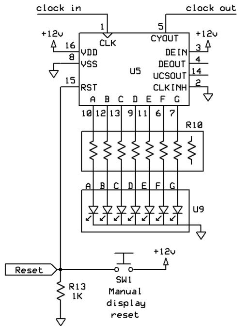
Like all CMOS chips, the counter chip (U5) has a limited ability to deliver output current. The datasheet states that the current which each output pin can supply when in the high voltage state (12 Volts) is typically about 6.8mA (at room temperature), but it can be as low as 3.4mA.
