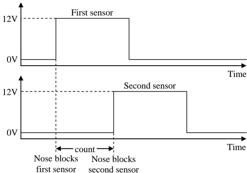
The output waveform of each sensor is high (12V) for as long as the passing slug keeps the light path interrupted. Since this measurement is done at the end of the barrel, the speed of the slug will be the same as it passes by both sensors (ignoring a bit of friction with the barrel which will slow the slug down), so the length of the two pulses should be the same. We are only interested in what happens when the nose
