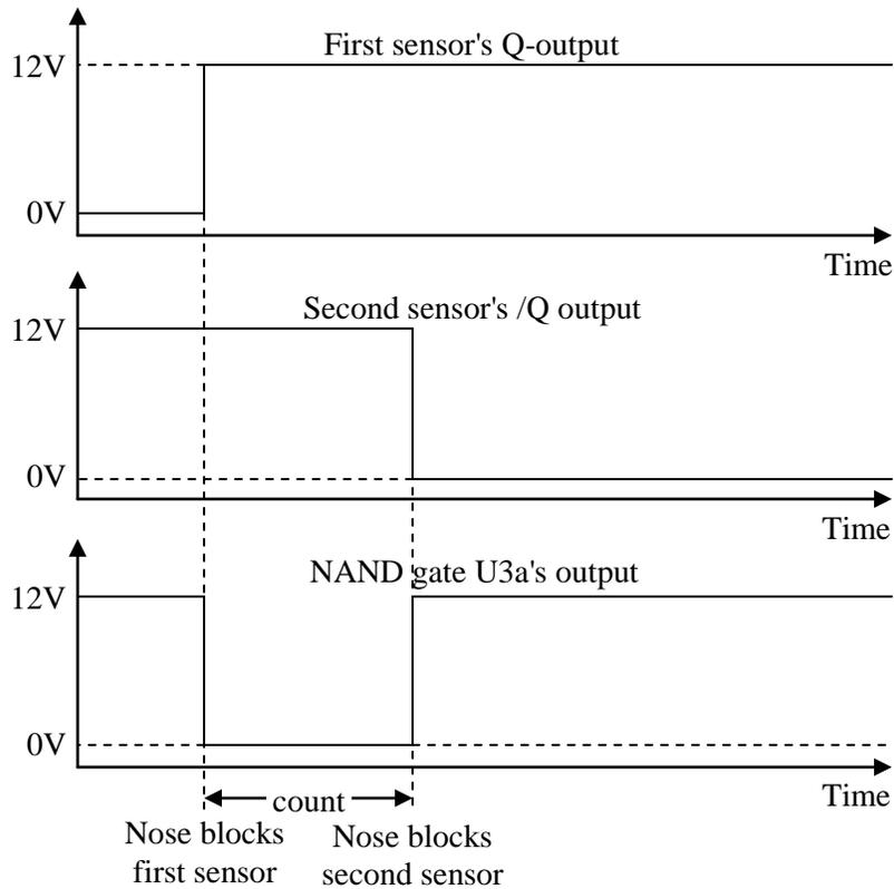
The output of NAND gate U3a is high except in the special circumstances when both of its input lines are high. In that case, and that case only, the output from U3a is low. NAND gate U3b inverts that negative pulse. And, it is during the high pulse from U3b that we want to count the 1MHz clocking pulses.
