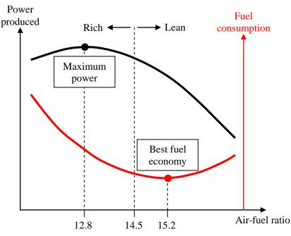
Running an engine at exactly its stoichiometric AFR makes it run very hot. Surprisingly, one of the most important results of running either lean or rich is that it reduces the temperature. In both settings, the mixture which passes through the cylinders includes unreacted gas – extra fuel in a rich mixture and extra air in a lean mixture – both of which carry away some of the heat.
