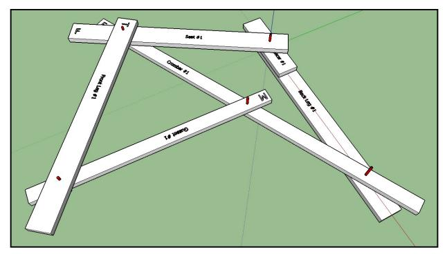
Since the frame is comprised of two independent triangles, it will fit together very nicely even if the holes were not drilled exactly where planned.
