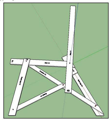
We are going to have to drill a hole near the bottom end of Back #1 so it can be pinned where the crossbar and gusset meet. To find out where to drill that hole, do the following. First, use a hammer or block of wood to tap down on the pin at the intersection of Crossbar #1 and Gusset #1. Tap the pin down so that its top is level with the surface of Gusset #1. Then, turn the entire assembly over.
