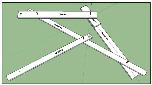
Next, Front Leg #1 is dropped onto the front pin as shown below, and the bottom holes of Front Leg #1 and Gusset #1 brought into alignment as shown by the red arrow.
