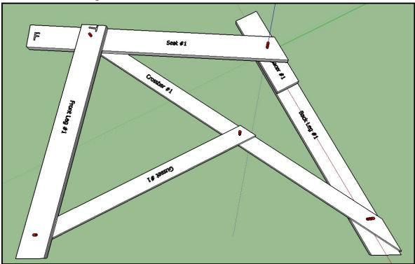
Now, let's begin the process of fitting Back #1. Start by sliding it down over the pin at the upper right, at the back of Seat #1.
