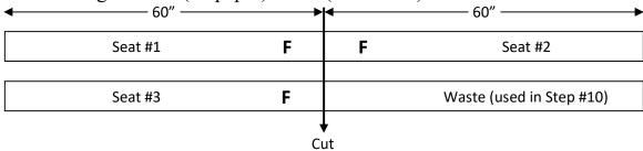
Step #5: Drill the following two holes (1/4-inch diameter) through the wide (6") face of each of the three Seats. The holes are centered across the width of the piece. Scale 1" (paper) = 20" (real).
