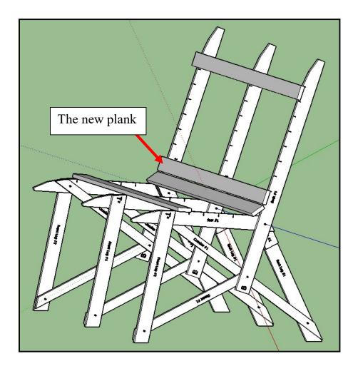
What we will do now is add two crossbars, oblique across the back, to help the bench resist "racking". The two planks already in place at the top and bottom of the bench's back lie in the same geometric plane, so attaching crossbars across them is not too hard.
