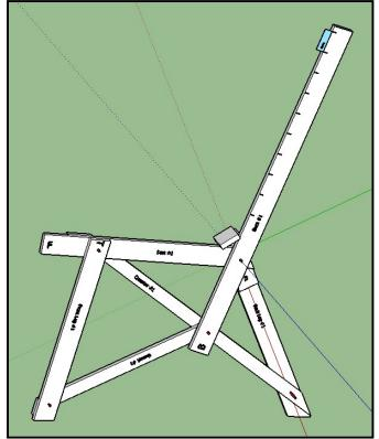
In the same way, make marks for the planks of the seat, starting with the IDEAL template snug against the scrap piece of 2" x 6".
