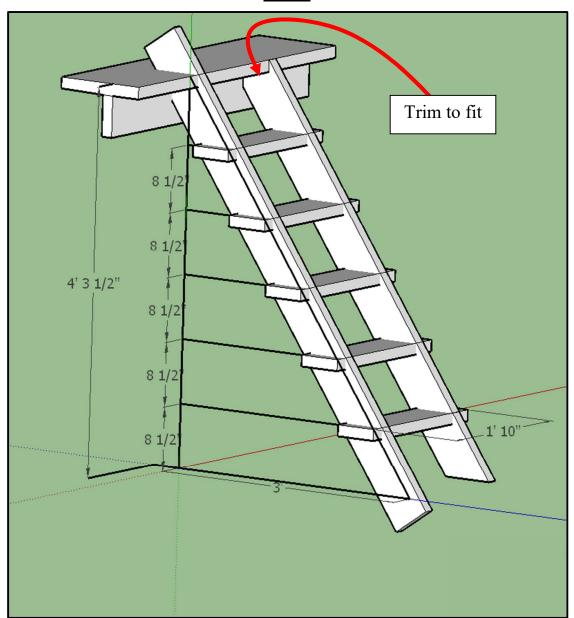
The stairs have an overall height of 4'3-1/2" from the ground to the top face of the seat planks. The stairs extend out 3' from the ends of the seat planks. The sides and treads are made from 2" x 6" planks. I have chosen the length and angle of the stairs so that each side can be cut from a six-foot length of 2" x 6" plank.
