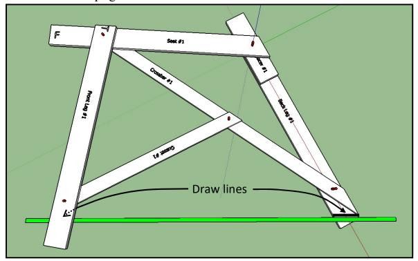
I placed the straight edge so that the scribed line across back leg passed about one-half inch below the intersection with the bottom side of the crossbar, and the scribed line across the front leg passed about one-half inch below the intersection with the bottom side of the gusset. The following figure shows what the frame will look like after the legs have been trimmed.
