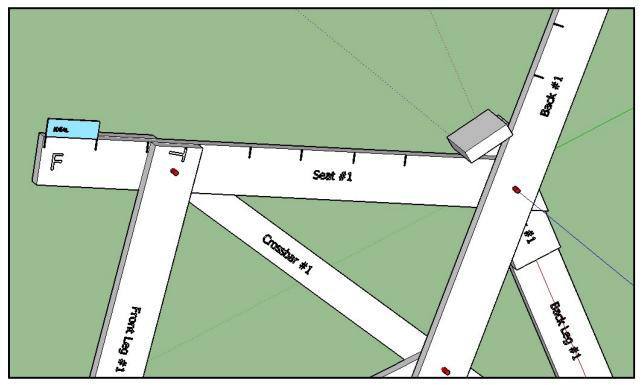
Although one could nail planks on to the back and seat at the locations now marked, the bench will be much more pleasing visually if the top of the back and the front of the seat are rounded off, and not left square. The following figure shows how the IDEAL 2" x 6" template can be used to round off Back #1.
