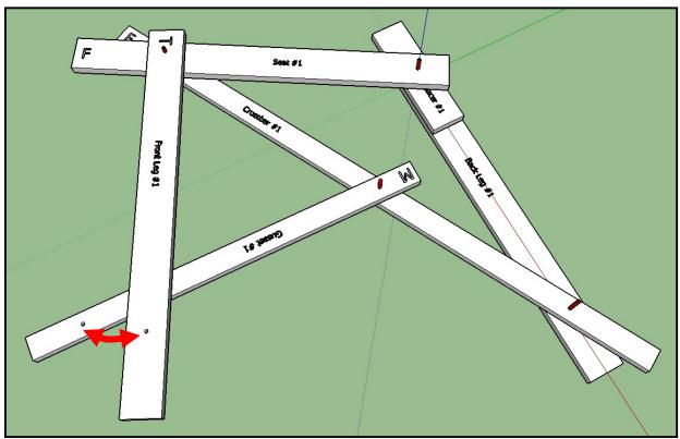
A final pin is driven through the aligned hole.
