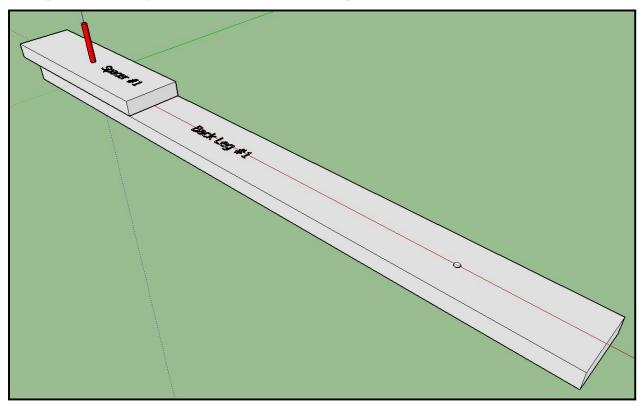
The red cylinder in the figure represents an eight-inch (or so) length of 1/4-inch threaded rod. Here, and again later, it is convenient to use such a rod to keep the holes lined up. If necessary, washers and nuts can be added to the ends to hold the assembly loosely together as it is moved around.
