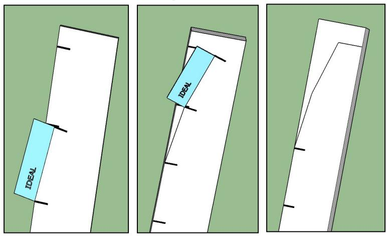
Three straight cuts will trim the top of Back #1 to a suitable shape. Do the same at the front of Seat #1, as shown next.
