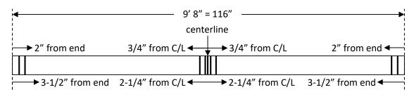
These nine lines are not intended to be guidelines for cutting. Instead, they will be used for aligning the planks when they are to be screwed to the frames. If a particular plank is to be mounted on the bench's seat, it should be aligned so that the three frames lie flat on the following red areas:
