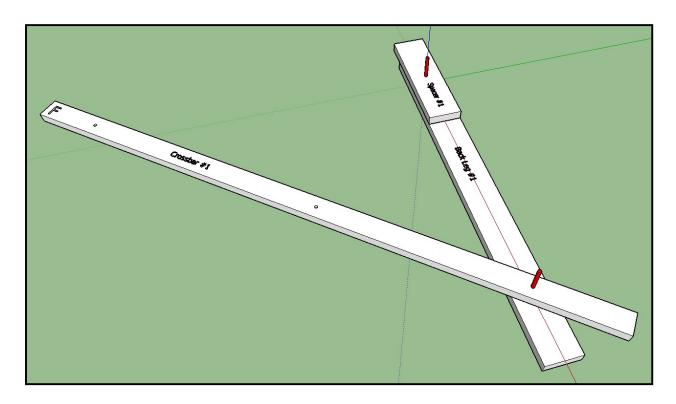
Now position Seat #1 so that its back hole slides down the top pin which comes up through Spacer #1. Note that Spacer #1 and Crossbar #1 are at the same vertical height (with respect to the surface of the page), so that Seat #1 will sit nice and flat on top of the two of them.
