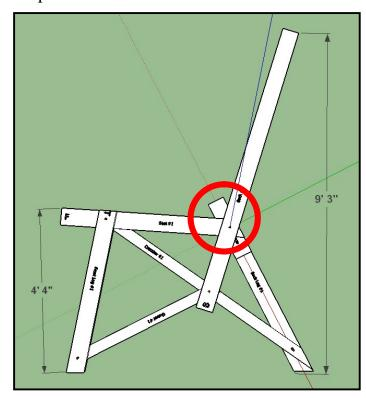
In the next Part, we are going to lay out the positions of the horizontal 2" x 6" planks that will be the seat and back of the bench. The purpose of this exercise is to determine how to trim the front end of Seat #1 and the top end of Back #1 for the best visual appeal. We will start the exercise by looking more closely at the junction shown inside the red circle shown to the left.
