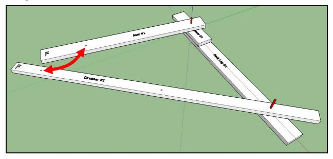
Now, pivot Seat #1 and Crossbar #1 around the two pins to bring their front holes into conjunction. The red arrow in the figure above shows the two holes to be
